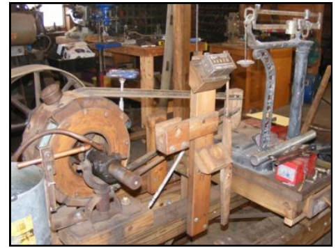
A Prony Brake at the Southland Flywheelers at their park in Hartselle, AL. Note the large brake to create load and the beam scale to measure pounds.
