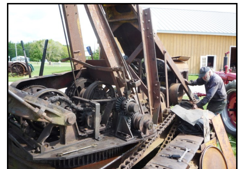
Bill Bartlett works on the 1926 Bay City Excavator. Where else can you see one?
