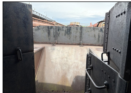
Not a very exciting photo, but behind the locomotive is the tender with its empty bin capable of holding 8 tons of coal. The top of the 5,000 gallon water tank can be seen in the rear. A strong back lad shovels coal to the locomotive's furnace while a pump moves water to its boiler.
