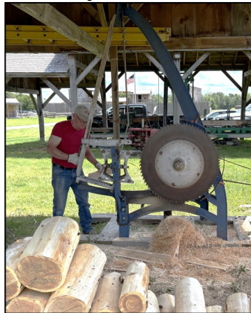
The team at the shingle mill made shingles to finish the Vertical Saw Mill roof.
