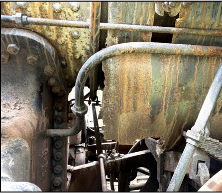
The Locomotive 210 boiler jacket (r) abuts the smoke box (l). Fasteners on the belly of the Jacket have rusted off, releasing it so it just hangs there. Asbestos insulation was inside the jacket, keeping the boiler hot. May 2026
